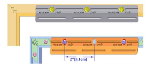
AMS Cleats are installed with screws on metal or wooden frames after assembly. Many widths are available to accomodate size and weight of frame. Locking option with additional hardware allows frames to be secured.
